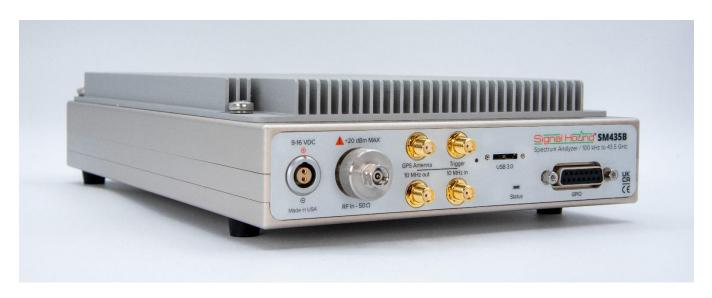
The SM435B is a high-performance spectrum analyzer and monitoring receiver. Tuning from 100 kHz to 43.5GHz, the analyzer has 160 MHz of instantaneous bandwidth (IBW), 110 dB of dynamic range, 1THz/sec sweep speed at 30kHz RBW (using Nuttall windowing), and ultra-low phase noise to rival even the most expensive spectrum analyzers on the market.
